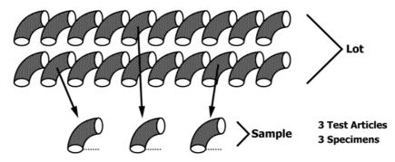
Each Specimen (5 or more measurements widely dispersed) must have Minimum Average Coating Thickness of (Table 1) -1 grade
